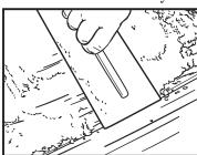
5. Allow cement mix to dry and install sheet water proofing membrane to manufacturer's specifications.
