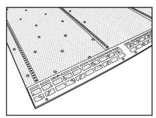
3.Attach Handie-Kirb to wood sub floors with 1" wood screws or  $1\ 1/2$ " tapcons screws on concrete sub floors.
